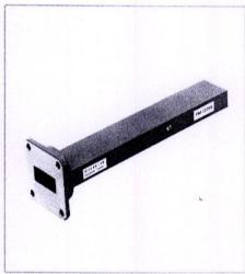
The low reflection termination PM 7220X has a very low VSWR and is designed for precision measurements. It is made of nickel-plated brass and finish is grey enamel.
