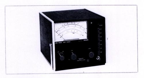
The SWR meter type PM 7833 is a lownoise 1000 Hz tuned amplifier/volmeter. To avoid hum caused by ground loop currents the measuring circuit is completely isolated from the mains ground.
