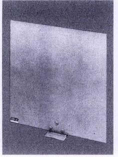
The microstrip antenna SL 19703 consists of a double-sided printed circuit board. One side forms the antenna pattern and the other a ground plane. The pattern is protected by a 10 mm thick layer of plexiglass. The pattern, consisting of an array of 16 patchs, is symmetrically excited. The antenna is fastened to an aluminium box which also serves as a support for the N-type coaxial contact.
