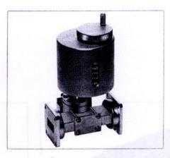
PM 7045X is a low power field displacement isolator. It is used in connection with oscillators to reduce load mismatches. The waveguide contains a magnetized ferrite bar to which a resistive plate is attached. Microwave energy travelling in the forward direction is very little attenuated. In the reverse direction the energy is absorbed in the resistive plate. This effect arises from the non-reciprocal distortion of the RF field caused by the magnetized ferrite.
