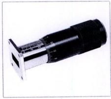
The standing wave detector PM 7142X consists of a straight waveguide section with a slot along the centreline of the broadslide wall, a probe carriage, a probe (antenna) inserted through the slot and a detector diode. The probe can be moved along the waveguide and the position is indicated on a mm-scale. The probe depth is adjustable. The microwave signal is coupled to the diode via the probe and the rectified signal behind the diode is fed to the BNC jack output on top of the detector mount.
